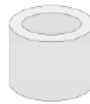
Image 20– Example of metal bushing that should be used to make the fixed points when the holes on the panels are all made with the same diameter as for the sliding points.
